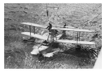
**Left**: FLGOFF John Napier Bell taxiing a Supermarine Seagull (Walrus) aircraft alongside the 'County' Class cruiser HMAS Canberra, for retrieval on completion of a flight following a catapult launch from the ship. (AWM).
